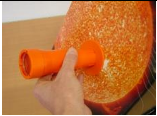
The tube is adjusted with a small counter clockwise rotation within grooves at different settings.
