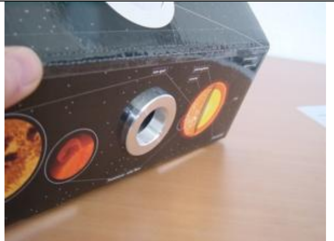
Step 7 The wide circular part of the mirror mount support n°8 must be positioned inner.
