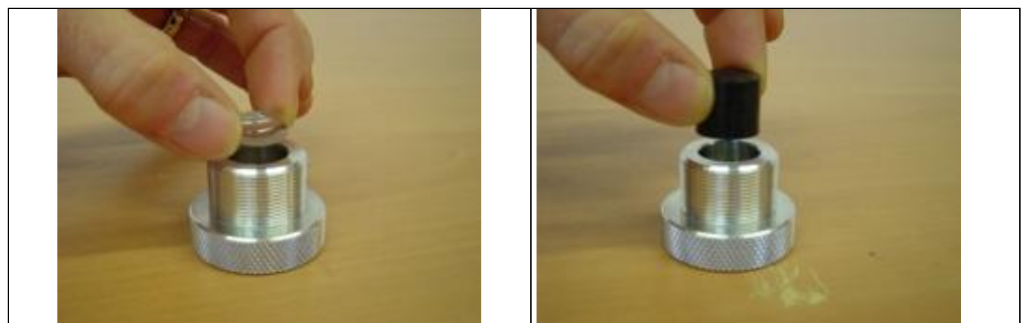
Put the mirror n° 11 into the mirror mount n° 9, the convex* side at the bottom
