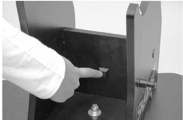
Figure 3. Position the rubber bumper "stop" over the index mark on the inside surface of the front brace.
