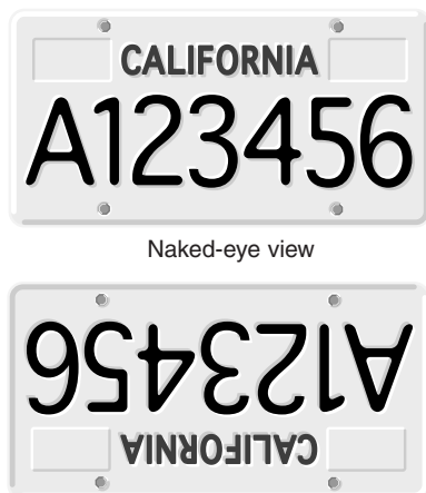
Figure 12. The view through a reflector telescope is upside down. This is true for the SkyQuest XT4.5. The view through the correct-image finder scope, however will be right-side up, oriented the same as seen with the naked eye.
