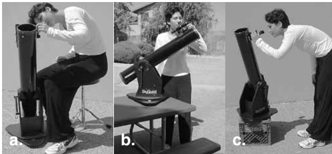
Figure 9: (a) Many people find the SkyQuest XT4.5 convenient to use while sitting. (b) You can use the telescope while standing by placing it on a sturdy table. (c) If the table is too tall, try something a bit shorter, like a milk crate.
