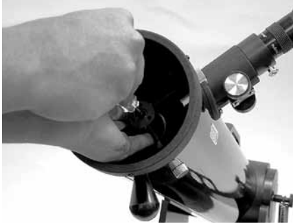
Figure 17. To center the secondary mirror under the focuser, hold the secondary mirror holder in place with your fingers while adjusting the center screw with the Phillips head screwdriver. Do not touch the mirror's surface.
