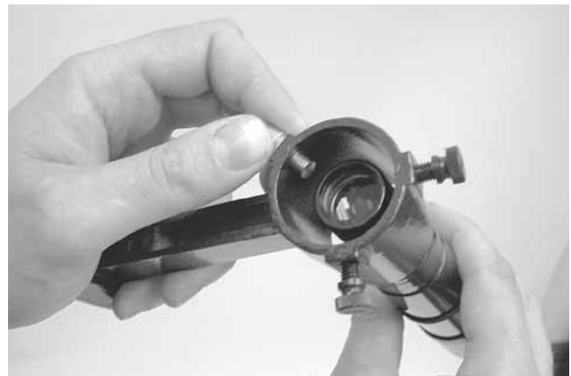
Figure 8b: Inserting the finder scope into the finder scope bracket
