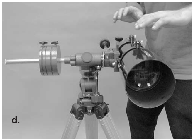
Figure 5. Proper operation of the equatorial mount requires that the telescope tube be balanced on both the R.A. and Dec. axes. (a) With the R.A. lock knob released, slide the counterweight along the counterweight shaft until it just counterbalances the tube. (b) When you let go with both hands, the tube should not drift up or down. (c) With the Dec. lock knob released, loosen the tube ring lock clamps a few turns and slide the telescope forward or back in the tube rings. (d) When the tube is balanced about the Dec. axis, it will not move when you let.
