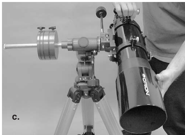
Figure 5. Proper operation of the equatorial mount requires that the telescope tube be balanced on both the R.A. and Dec. axes. (a) With the R.A. lock knob released, slide the counterweight along the counterweight shaft until it just counterbalances the tube. (b) When you let go with both hands, the tube should not drift up or down. (c) With the Dec. lock knob released, loosen the tube ring lock clamps a few turns and slide the telescope forward or back in the tube rings. (d) When the tube is balanced about the Dec. axis, it will not move when you let.
