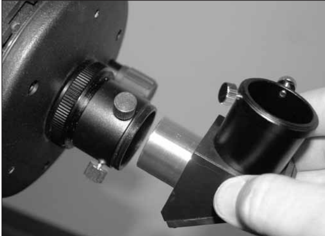
Figure 8. Attaching the star diagonal (refractor and Maksutov-Cassegrain models only).
