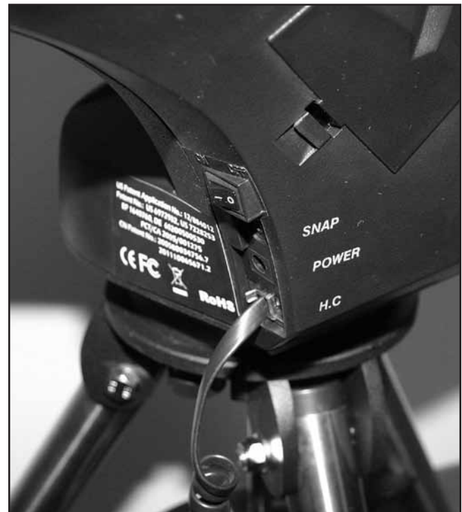
Figure 16 The electronic ports for the hand controller and an optional 12V DC battery are located at the base of the mount arm. The SNAP port allows control of a DSLR camera when used with proper cable.
