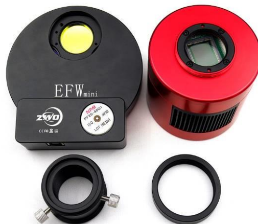
Screw off the T2-1.25" holder on the EFW, screw off the T2 ring on the 1600-C.
