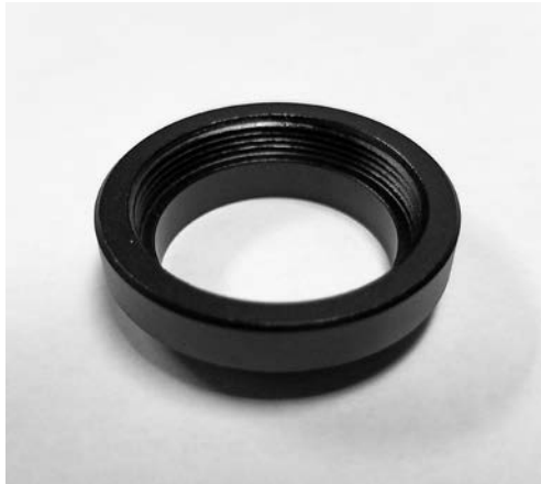
Figure 4. The CS/C Extension Ring is needed to couple CS-mount cameras to the 30mm Ultra-Mini Guide Scope, in order to achieve proper focus.
