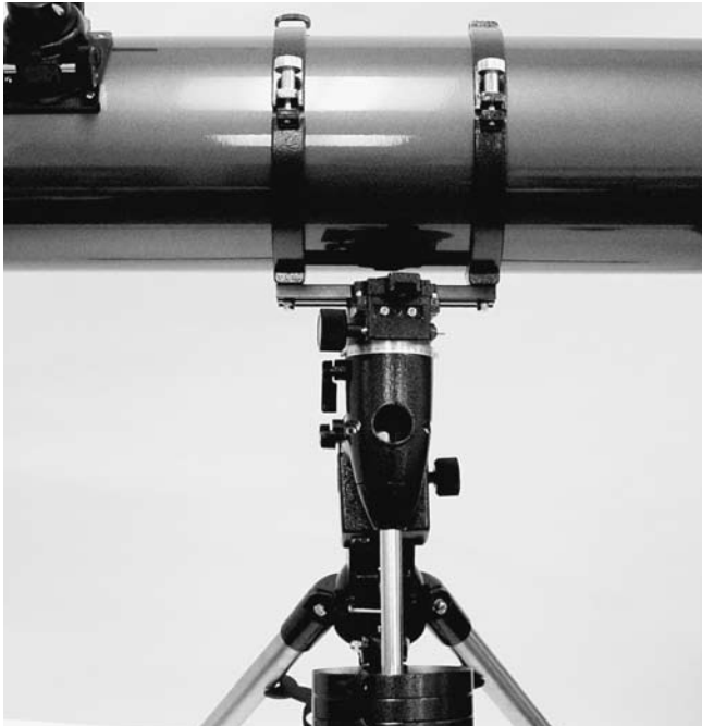
Figure 8. The optical tube must be at a 90° angle to the right ascension axis in order to view through the polar axis finder
